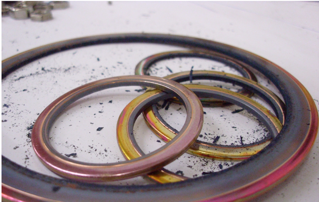
Figure 5.1: Photograph showing the corrosion of copper gaskets caused by sulfur in the growth chamber before their replacement with Ag-plated gaskets.
