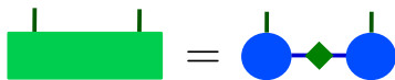
Figure 2.3: Singular value decomposition: When regarding two neighbouring sites, the correlation between the particles on the sites can be measured via the singular value decomposition. The matrix connecting site i and i+1 is diagonal; the entries are the singular values. Their amplitudes are a measure for the correlation between the particles in the system.
