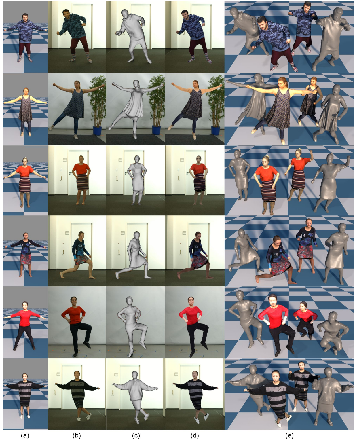
Fig. 5. Qualitative results. We show several live monocular performance capture results of entire humans in their loose everyday clothing. (a) shows the template models. (b) shows input images to our method, while (c) shows that the corresponding results precisely overlay the person in the input images. Our results can be used to render realistic images (d) or free viewpoint video (e).
