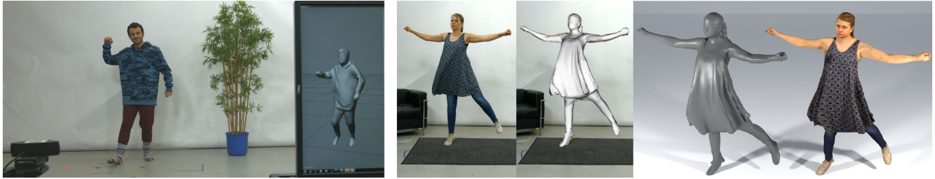
Fig. 1. We propose the first real-time human performance capture approach that reconstructs dense, space-time coherent deforming geometry of people in their loose everyday clothing from just a single monocular RGB stream, e.g., captured by a webcam.
