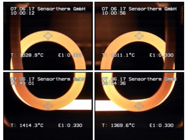
Fig. 6: Snapshots from the pyrometer camera taken during temperature measurements of different parts of the filament (heating current is 20 A).
