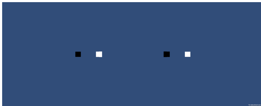
FIGURE 3.8: SSVEP stimulus used for the testing procedure to identify the settings to produce a stable flickering on the head mounted display screen. There are only two blinking boxes, the other two are due to stereoscopic imaging to produce a three dimensional perception.
