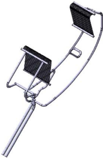
Fig. 2. PFCs cooling circuit layout option 2 (Rev A).
