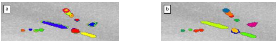
Figure 4. Close up to a cluster of hot spots on tile 6 at filter version 0 (a) and the chosen filter version 3 (b), at the threshold of 180 and min_persistence at 4. With the version 0, the area is covered by 42 catalogue hot spot entries, while in the version 3 the number is reduced to 15.
