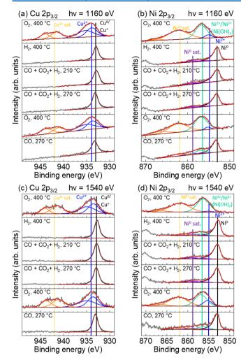
**Figure 3.** NAP-XPS spectra of the Cu  $2p_{3/2}$  (a, c) and Ni  $2p_{3/2}$  (b, d) core level regions of CuNi NPs on SiO<sub>2</sub>/Si(111) acquired *in situ* in different gases (at a pressure of 0.4 mbar for the pure gases and 0.48 mbar for the reactant mixture) at the temperatures indicated on the graphs. X-ray photon energies of (a, b) 1160 eV and (c, d) 1540 eV were used for acquiring the depth profiles of the NPs.
