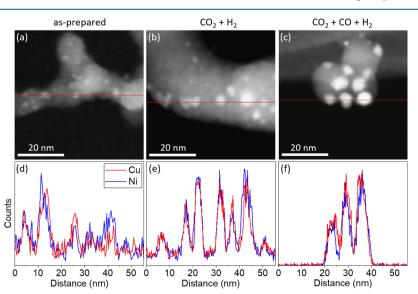
Figure 2. STEM images of a  $Cu_{0.5}Ni_{0.5}/SiO_2$  powder catalyst obtained (a) before the catalytic reaction, (b) after catalytic reaction in  $CO_2 + H_2$  (vol. 1:3) and (c) after catalytic reaction in  $CO_2 + CO + H_2$  (vol. 4.5:11.5:84) at 20 bar (210–270 °C). EDS linear scans (d-f) show the relative amounts of Cu (red) and Ni (blue) along the lines shown in the respective STEM images in the upper row.
