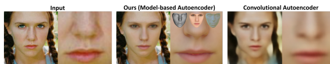
Fig. 16. Our model-based autoencoder gives results of higher quality than convolutional autoencoders. In addition, it provides access to dense geometry, reflectance, and illumination.
