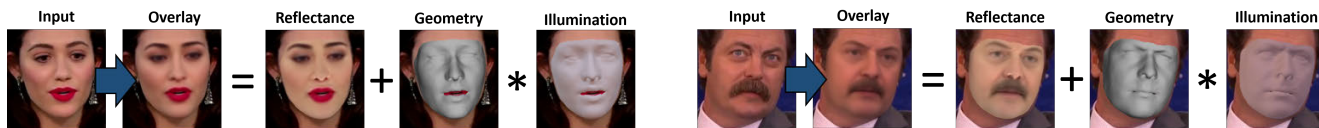
Figure 1. We propose multi-frame self-supervised training of a deep network based on in-the-wild video data for jointly learning a face model and 3D face reconstruction. Our approach successfully disentangles facial shape, appearance, expression, and scene illumination.
