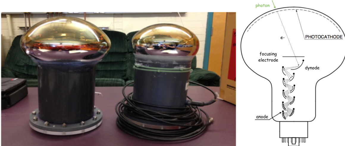
Figure 2.3: Left panel: PMTs used in HAWC (left: 10", right: 8"). Right panel: Schematic diagram of a typical PMT. The PMT schematic is taken from (Wood 2018).
