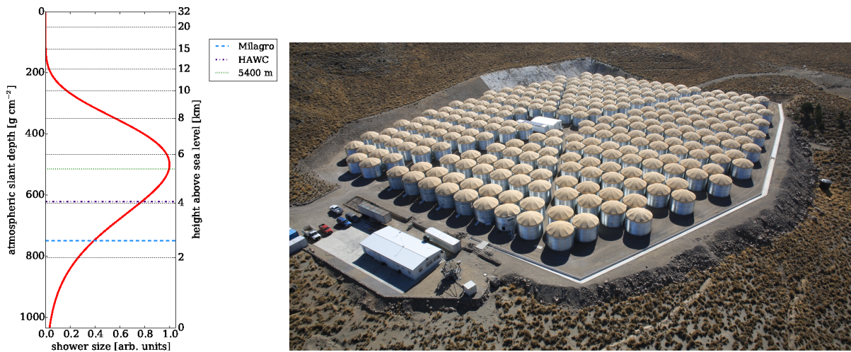
Figure 2.1: Left panel: shower size as a function of the depth travelled in the atmosphere and height a.s.l.. Right panel: The complete HAWC \gamma -Ray Observatory. Showing all the WCDs, the counting-house at the center and the utility building at the bottom left corner. The plot on the left panel is taken from (BenZvi 2018).
