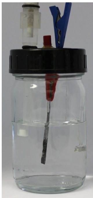
Figure S2. Cell used for electrochemical experiments.
