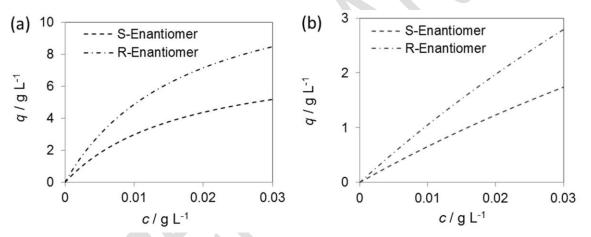
Figure 3. Single component Langmuir adsorption isotherms of: (a) Isoflurane enantiomers; (b) Desflurane enantiomers. S corresponds to component 1 and R to component 2 for both substances. Isotherm parameters were determined at 28 °C and are given in Tab. 2.
