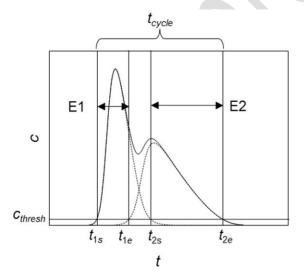
Figure 1. Representation of a racemic mixture elution profile with marked cycle time, threshold concentration ( $c_{thresh}$ ) and four characteristic cut times ( $t_{1s}$  and  $t_{1e}$  for enantiomer 1 and  $t_{2s}$  and  $t_{2e}$  for enantiomer 2), between which the pure enantiomers (E1 and E2) are collected.
