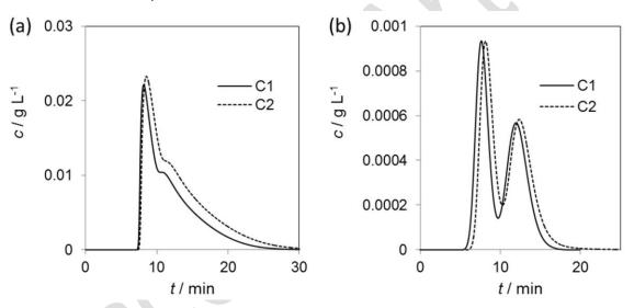
Figure 7. Experimental validation of the scale-up procedure illustrated by comparison of the experimental elution profiles for two columns: (a) Isoflurane – C1 (d = 0.6 cm, flowrate 71 mL min<sup>-1</sup>,  $V_{inj}$  = 5 µL) and C2 (d = 1.56 cm, flowrate 492 mL min<sup>-1</sup>,  $V_{inj}$  = 40 µL); (b) Desflurane – C1 (d = 0.6 cm, flowrate 21 mL min<sup>-1</sup>,  $V_{inj}$  = 0.04 µL) and C2 (d = 1.56 cm, flowrate 152 mL min<sup>-1</sup>,  $V_{inj}$  = 0.4 µL).
