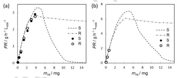
Figure 5. Dependency of the productivity of: (a) Isoflurane; (b) Desflurane enantiomers (S and R) on the injected amount of one enantiomer. The volumetric flowrate was 71 mL min<sup>-1</sup> for isoflurane and 21 mL min<sup>-1</sup> for desflurane. Lines represent the results from the simulation study and symbols the values estimated from the experiments.
