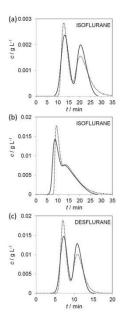
Figure 4. Comparison of the experimental (dotted line) and simulated (solid line) elution profiles for different injection volumes: (a) Isoflurane 1  $\mu$ L (0.75 mg of one enantiomer); (b) Isoflurane 5  $\mu$ L (3.84 mg of one enantiomer); (c) Desflurane 1  $\mu$ L (0.70 mg of one enantiomer). Pure racemic mixtures were injected in the liquid phase. The flowrate was 71 mL min<sup>-1</sup> for isoflurane experiments and 21 mL min<sup>-1</sup> for desflurane.
