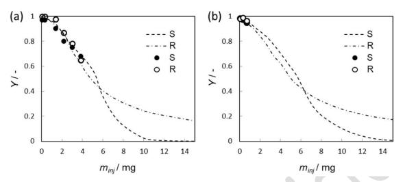
Figure 6. Dependency of the recovery of: (a) Isoflurane; (b) Desflurane enantiomers (S and R) on the injected amount of one enantiomer. The volumetric flowrate was 71 mL min<sup>-1</sup> for isoflurane and 21 mL min<sup>-1</sup> for desflurane. Lines represent the results from the simulation study and symbols the values estimated from the experiments.
