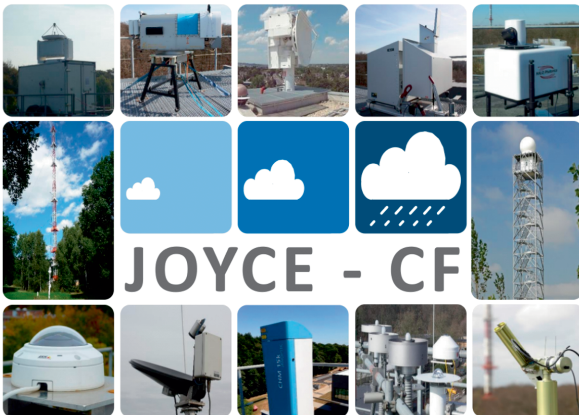
Fig. 2. Instrumentation of Supersite JOYCE-CF. (top, from left to right): MIRA 35-GHz cloud radar, HATPRO microwave radiometer, BoXPol radar, AERI infrared interferometer, and Doppler wind lidar. (middle) 120-m-tall tower with meteorological sensors, and JuXPol radar. (bottom, from left to right): Total sky imager, micro rain radar, ceilometer, solar and terrestrial radiometers, and sun photometer. All instruments except JuXPol (at Sophienhöhe) and BoXPol (in Bonn) radars are located at the Research Center Jülich.
