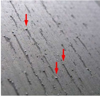
Figure 7: Photograph showing delamination of W coating on outer divertor tile.
