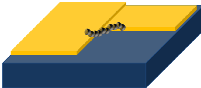
Figure 2.16 Sputtered pattern on the SEM substrate. The magnetosomes are placed on the cross section of the layers.
