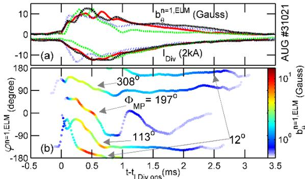
Fig. 4 (color online). The evolution of (a) the amplitudes and (b) the toroidal phases of the  $n = 1$  component of NAMPs for the four ELMs shown in Fig. 3.  $b_\theta^{n=1,\text{ELM}}$  is also indicated by the color scale in (b). The time with respect to the ELM onset ( $t_{1,\text{Div,ons}}$ , as marked in Fig. 3) are used.
