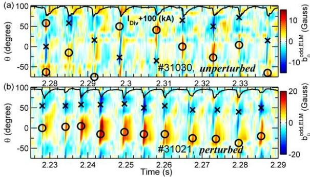
Fig. 2 (color online). Comparison of the poloidal distribution of  $b_\theta^{\text{odd,ELM}}$  for the (a) *unperturbed* and (b) *perturbed* plasmas by the  $n = 1$  MP field. The tile currents measured in the outer divertor,  $I_{\text{Div}}$ , are plotted in black lines as an indicator of the ELM crashes. The circles and crosses mark the peaks and dips of NAMPs respectively.
