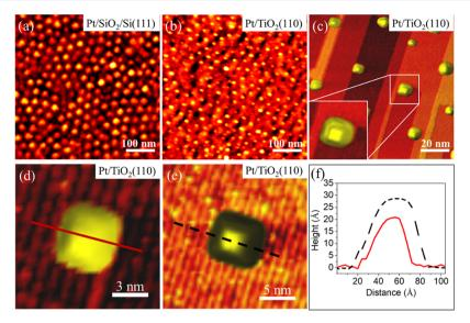
Figure 1. (1 × 1 μm) AFM images of the as-prepared Pt NPs supported on (a) SiO<sub>2</sub>/Si(111) and (b) TiO<sub>2</sub>(110). (c-e) STM images of polymerfree Pt NPs on TiO<sub>2</sub>(110) acquired at 25 °C after annealing in vacuum at 1100 °C. The inset in (c) and the high-resolution images in (d,e) display truncated octahedron Pt NPs on TiO<sub>2</sub>(110) with (100) top and interfacial facets. (f) Line profiles of the Pt NPs, shown in (d,e).
