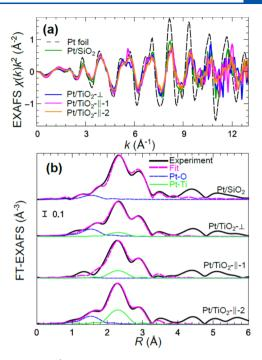
**Figure 3.** k-space  $k^2$ -weighted Pt L<sub>3</sub>-ege EXAFS data (a) and Fourier-transformed EXAFS data (b) for Pt NPs on SiO<sub>2</sub> and TiO<sub>2</sub>(110). Fitted spectra considering Pt—Pt and Pt—O bonds for NPs on SiO<sub>2</sub>/Si(111), and Pt—Pt, Pt—O, and Pt—Ti bonds for NPs on TiO<sub>2</sub>(110) are also shown. For clarity, spectra are shifted vertically in (b).
