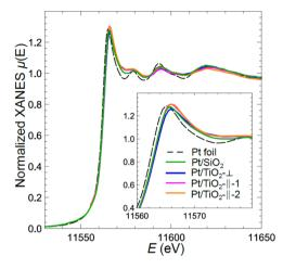
**Figure 2.** Experimental Pt  $L_3$ -edge XANES spectra measured at 25 °C in UHV corresponding to Pt NPs supported on SiO<sub>2</sub> and TiO<sub>2</sub>(110). The data on TiO<sub>2</sub> were acquired in three different X-ray polarizations, two parallel to the support surface and one perpendicular. Data from Pt foil are also shown for reference.
