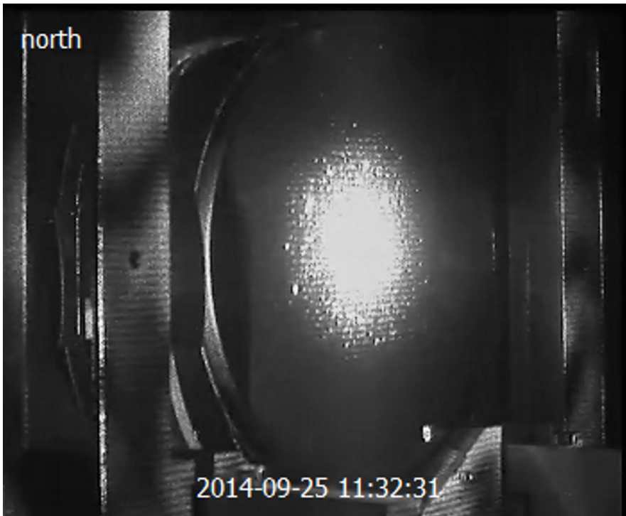
Figure 2.11.: This image (taken with camera that is sensitive to the laser wavelength of 1064 nm) shows the highly reflective front surface of the north folding mirror. The bright spot on the mirror is caused by the laser beam. Laser light is scattered from the mirror surface into the camera. High order modes extending beyond the mirror edge can be seen as well. They illuminate spots on the metal bars left and right of the mirror, as well as the catcher underneath the mirror. Furthermore, the ‘illuminated’ parts in the image show a pattern of horizontal stripes, with a spacial period of 2-3 mm, compared to the mirror diameter of 180 mm. The stripes are produced by the interference of two beams hitting the mirror at an angle, which is discussed in detail in [HCG + 14].
