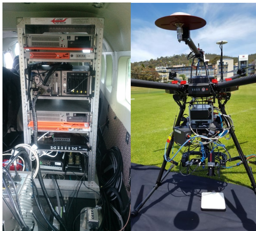
Figure 5. Two different F sensors installed on different platforms: HyPlant installed in an aircraft (left) and AirSIF system with QE pro of the Terraluma group installed on a multirotor UAV (right).
