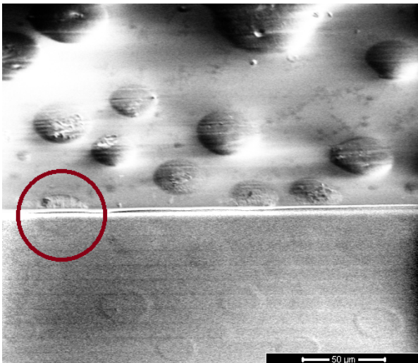
Figure 7.3: The lower half exposed to the ion beam is separated by a sharp line. Red marked is a bubble where half of it was exposed and the other protected. The original SEM image was edited (software GIMP) so that the lower half shows clearer contrast.
