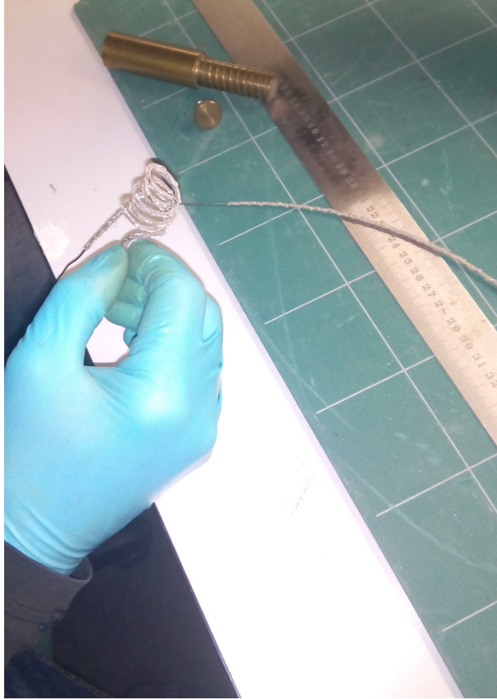
Figure 4.5: Coiled ion source filament before coating. In the background, the grooved brass cylinder used to coil the filament and an uncoiled tantalum filament, already wrapped in a nickel mesh, can be seen.
