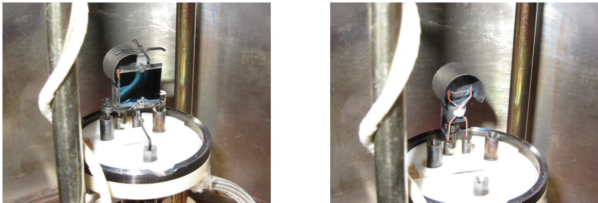
Figure 4.14: Target platform with heating filament, with (left) and without target (right). The two hind legs of the target holder are connected to a type-K thermocouple. The front leg is connected to a power supply which sets the bias of the sample. The heating cup is electrically connected to the heating filament. The hooks situated on top of the target holder are used to weigh the sample and to transport it between target chamber, load-lock and TDS chamber.
