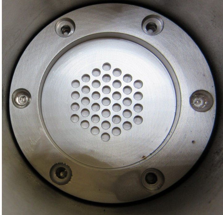
Figure 4.6: Ion source extraction grid with partly-melted steel screws. The screw heads have either melted or have broken off due to thermal stresses.
