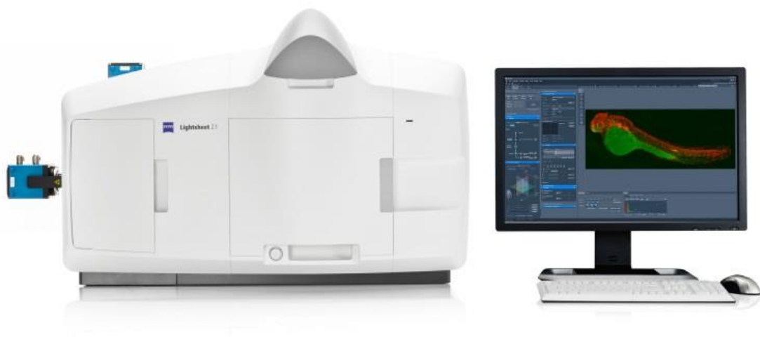
Figure 6 Set-up of the Light-Sheet-Fluorescence-Microscope Z.1 manufactured by Zeiss with an example of an imaged zebra fish on the monitor[20].
