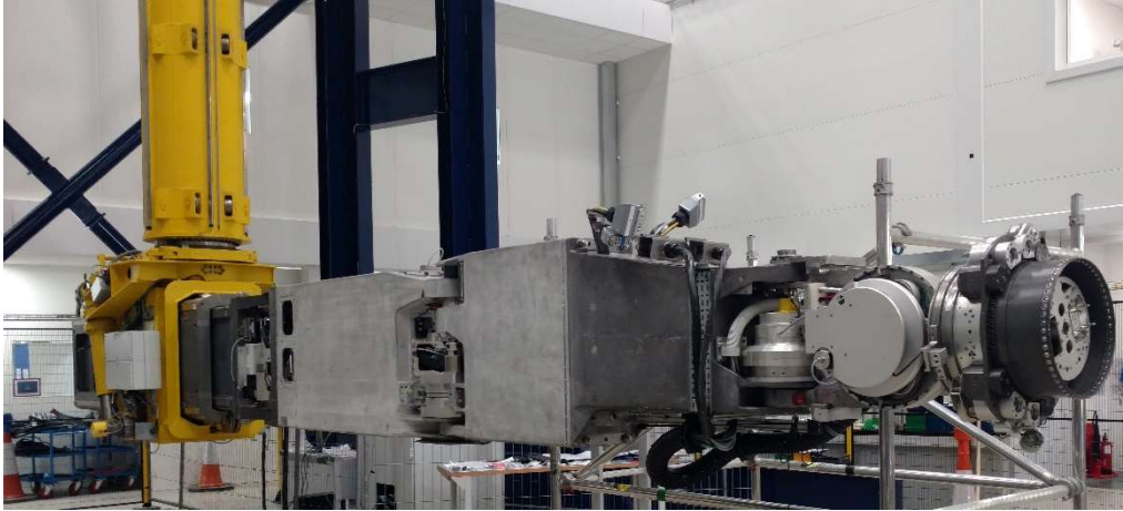
Figure 12 - Refurbished TARM manipulator mounted from new deployment frame
