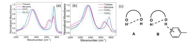
Figure 4. IR spectra of ~ 100 mM (a) 1nTADDOL and (b) 2nTADDOL in different solvents. The absorption due to the solvent was subtracted and spectra were normalized to the maximum absorbance at 3300-3400 cm<sup>-1</sup>. (c) Scheme of the intramolecular hydrogen-bond (A) and the intermolecular hydrogen-bond to aromatic solvents like e.g. toluene (B).
