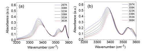
Figure 5. Background-subtracted IR spectra of ~150 mM (a) 1nTADDOL and (b) 2nTADDOL dissolved in toluene as a function of temperature.
