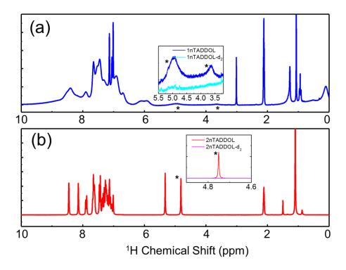
Figure 2. <sup>1</sup>H NMR spectra of ~30 mM (a) 1nTADDOL, and (b) 2nTADDOL dissolved in toluene-d<sub>8</sub> at 298 K. The peaks at 2.1, 7.0 and 7.1 ppm are due to residual protons of toluene. The insets show the comparison of (a) 1nTADDOL and 1nTADDOL-d<sub>2</sub> and (b) 2nTADDOL and 2nTADDOL-d<sub>2</sub> for the OH proton signals \*
