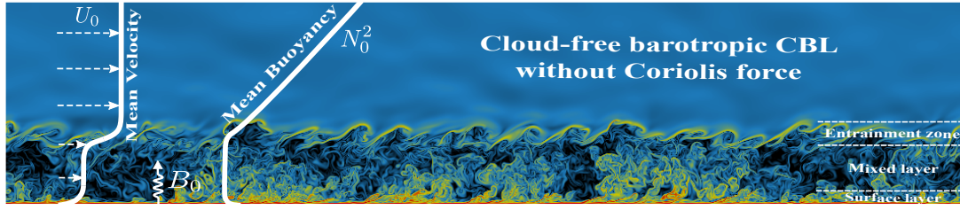
Figure 2: Sketch of the cloud-free barotropic CBL in the quasi-steady regime considered in this work. The background is a cross-section of the logarithm of the magnitude of the buoyancy gradient for a strongly sheared CBL.
