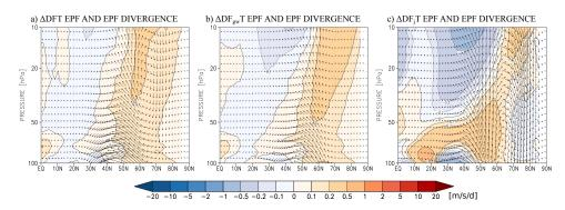
**Figure 3.2.**  $\Delta DFT$ ,  $\Delta D_{gw}FT$  and  $\Delta D_jFT$  lower stratospheric zonal wind tendency due to EP-flux divergence shown in color shading [m/s/d]. Arrows show the EP-flux change. The Arrow size is scaled in order to fit visual properties.
