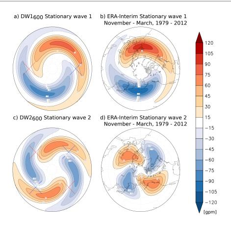
**Figure 2.8.** Polar stereographic plot of the filtered stationary wavenumber 1 (upper row) and stationary wave number 2 (bottom row) at 500hPa. a) shows the DW1<sub>600</sub> control experiments and c) the DW2<sub>600</sub> control experiments. b) and d) show ERA-Interim Northern hemisphere stationary waves. Red crosses denote maxima and blue crosses minima of the sinusoidal anomaly in the geopotential height.
