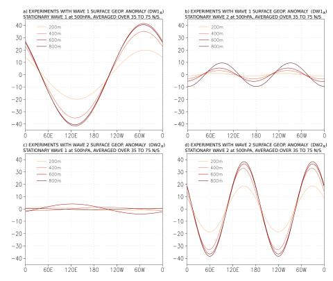
**Figure 2.7.** Stationary wave amplitudes at 500hPa for different surface geopotential height anomalies. a) and b) show control experiments with a forced stationary wave number 1. c) and d) show control experiments with a forced stationary wave number 2. The left column shows the filtered stationary wave number 1 and the right column the filtered stationary wave number 2.
