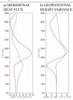
**Figure 3.7.** Mean integrated meridional heat flux change shown in a) and mean integraded geopotential height variance change shown in b). The integration is performed over wavenumber 1 to 12. The red line shows the  $\Delta D_j$ FT change and the blue line the  $\Delta MF4K$  change.
