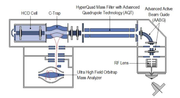
Figure 5 Functional elements in the Q Exactive HF mass spectrometer<sup>57</sup>.
