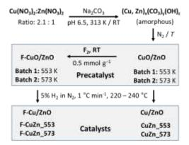
**Figure 1.** Synthesis routes to the four catalysts used in this study. Those that were oxidatively fluorinated by  $F_2$ , carry the label "F-"; and the number after "CuZn\_" gives the calcination temperature in K.
