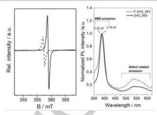
Figure 3. Left) X-band EPR spectra of the fluorine treated ZnO sample (solid) and its counterpart (dashed). Right) Normalized photoluminescence spectra of the fluorine treated ZnO sample (dashed) and its source sample (solid). F-content of sample F-ZnO: 1.2±0.1 wt.%
