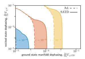
FIG. 5. Comparison of the smallest gate error between adiabatic and accelerated gates. For fixed values of the dephasing rates we look for the gate time that yields the smallest error. We consider an uncertainty on  $\Omega_0$  of 10% (k=0.05) and  $\Gamma_{\varphi,0}=\Gamma_{\varphi,1}=\Gamma_{\varphi,a}=\Gamma_{\varphi,GS}$ . The accelerated gate reaches the same error as the adiabatic gate for dephasing rates that are roughly one order of magnitude larger.
