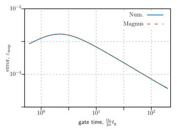
FIG. 6. Comparison of the average error  $\varepsilon_{\rm map} = 1 - \bar{F}_{\rm map}$  calculated numerically (solid blue trace) vs using Eq. (49) (dashed orange trace). We used  $\alpha = \pi/4$ ,  $\beta = 0$ ,  $\gamma_0 = \pi$ ,  $\Gamma_{\varphi,e} = \Omega_0/(2\pi \times 100)$ .
