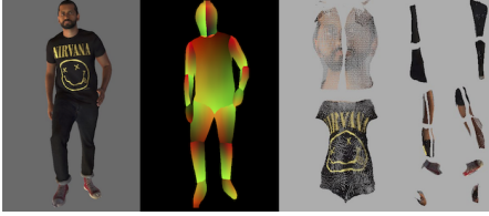
Figure 3. To create the input to our method, we first process the input image (left) with DensePose. The DensePose result (middle) contains UV coordinates, that can be used to map the input image into a partial texture (right).
