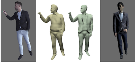
Figure 7. After training with MS-DSSIM loss enabled (green) complex clothing is reconstructed more reliably, than after training with L1 loss only (yellow).
