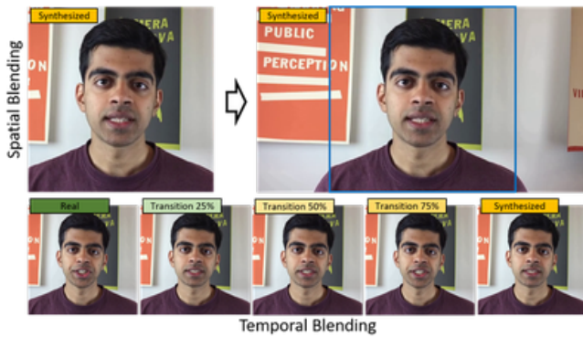
Fig. 11. Our approach enables us to seamlessly compose the modified segments back into the original full frame input video sequence, both spatially as well as temporally. We do this by explicitly conditioning video generation on the re-timed background video.
