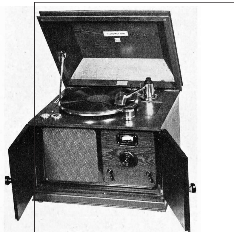
FIG. 1 “A playback machine with an electrical (sound amplification) box, connected with radio reception.” (Source: Doegen, Jahrbuch des Lautwesens 1931, 122.)
