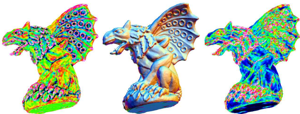
Figure 3: Color encodings for the mean curvature (left) and curvedness (right) detected on Gargoyle model (center).
