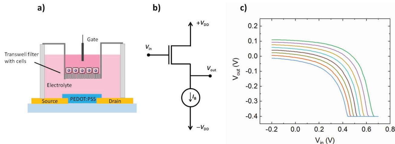
**Figure 2.** OECT as a sensor for cell barrier integrity: a) Device structure with an integrated Transwell filter with cells.<sup>[25]</sup> b) Schematic circuit of the current-driven configuration. c) Measured transfer characteristics of a current-driven OECT for  $I_B$  ranging from  $-0.7$  till  $-1.4$  mA (top to bottom) at  $V_{DD} = 0.2$  V. Device dimension were  $W = 2$  mm,  $L = 1$  mm. A Ag/AgCl gate electrode and EMEM cell culture medium as an electrolyte was used.
