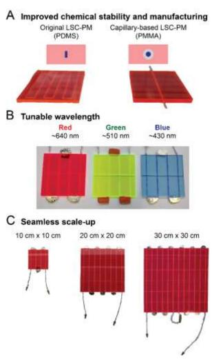
**Figure 1.** (A) Photographs and schematic comparison between the capillary-based LSC-PM (right) and the original design (left); (B) photographs of LSC-PMs with different dye dopants; (C) LSC-PMs of different sizes, with irradiated volumes of 177  $\mu$ L, 707  $\mu$ L and 1.59 mL respectively.
