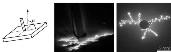
Fig. 2. Scheme of the inclined cathode arrangement showing the emission angle \alpha (left), open-shutter photographs of the cathode during a discharge (current 0.5 kA, duration 1 ms) through a window (middle) and vertical open-shutter photograph of a discharge with 1 kA / 0.5 ms showing the radiation along the arc traces, taken earlier in another experimental device (right)
