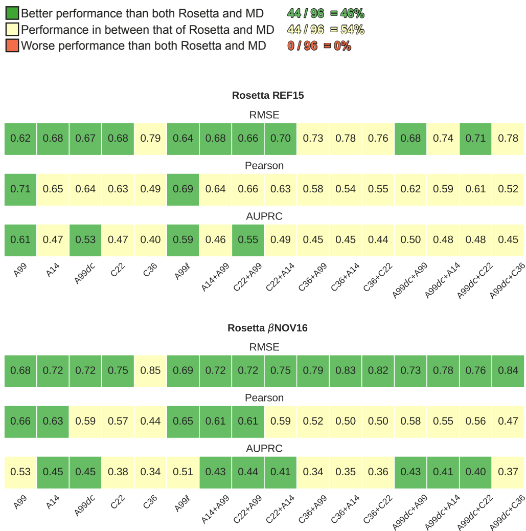
Figure S7: Results obtained with a combined Rosetta and MD consensus approach[56]. Each cell shows the performance of the consensus results obtained by averaging the results from Rosetta (REF15 scoring function at the top, \beta NOV16 function at the bottom) and the free energy calculations (abbreviations as defined in Table S1; the use of two abbreviations, e.g. “A14+C22”, denotes a consensus force field result). Cells are color-coded depending on whether the performance of the consensus approach was better, in between, or worse than the performance of Rosetta or MD alone.
