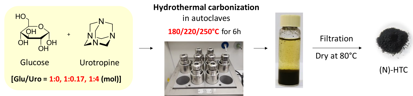
Scheme 1. Synthetic Scheme of the Hydrothermal Carbonization for Different Amounts and Types of N-Functional Groups Using Glucose and Urotropine as Precursors
