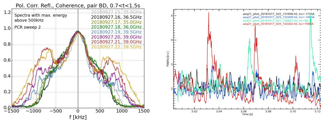
Fig.5 Mode activity detected by the correlation reflectometry system (left) and change of the mode activity in discharges with different island size (right).
