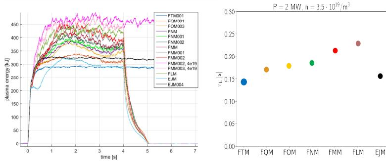
Fig.3 Diamagnetic energy and confinement time in configuration scans.
