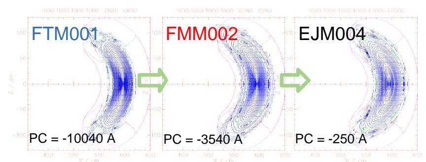
Fig.1 Poincaré plots for the scan between high iota (FTM001) and standard (EJM004) configurations.
