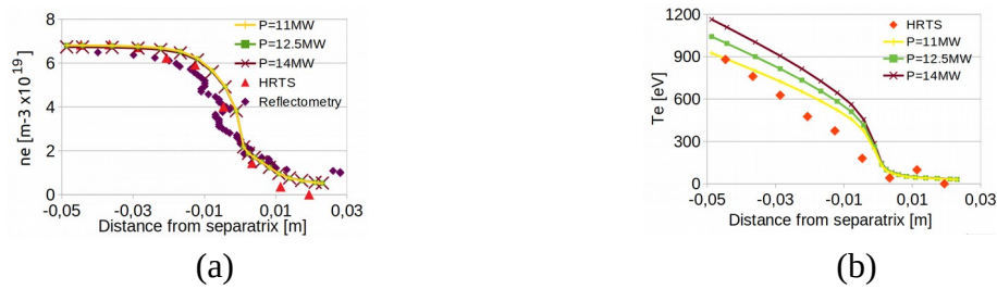
Figure 2: Upstream profiles of n_e (a) and T_e (b) with the new set D, X compared with HRTS (red triangles) and reflectometry (purple diamonds) data of the JPN 85419 at t = 18s mapped on the outer miplane .
