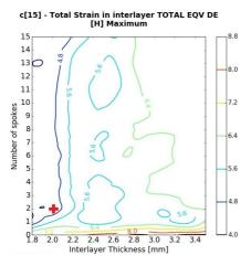
Fig. 6. Example of a single response surface for a given parameter – total strain in the interlayer. Red cross indicates Phase 2 design selection.
