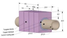
Fig. 4. Summary of geometric constraints in mm for  $2^{nd}$  phase mock-ups (agreed within EUROfusion WPDIV). The design optimization took these dimensions as fixed.
