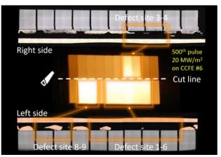
Fig. 1. CCD camera image of mock-up #6 under 20 MW/m<sup>2</sup> at GLADIS (IPP, Germany). Displayed on the top and bottom of the image are microscope images of the axial cross-section. Defect sites 3-4 on the right side, and defect sites 1-6, 8-9 on the left side match the observation of overheated blocks during the mock-up test.
