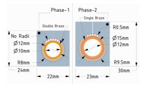
Fig. 5. Phase 1 monoblock compared to Phase 2 monoblock design.
