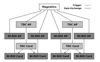
Figure 2: Illustration of the internal AP structure of the DCS satellite for the new magnetics on ASDEX Upgrade. The APs are indicated by the grey rectangles, the hardware is indicated by the grey boxes with rounded corners.
