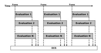
Figure 5: Illustration of the VRT evaluation timing. All evaluations for a camera are executed when a new frame has been acquired. The result for each evaluation is send to DCS as soon as it becomes available.
