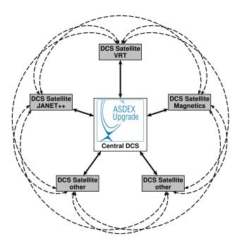
Figure 1: Illustration of DCS satellites communication with central DCS. The real time data and configuration communication is shown as bold arrows, the real time data only communication is shown as dashed arrow. Offline data storage is handled by the data management system at ASDEX Upgrade [17] and is not illustrated in this figure.
