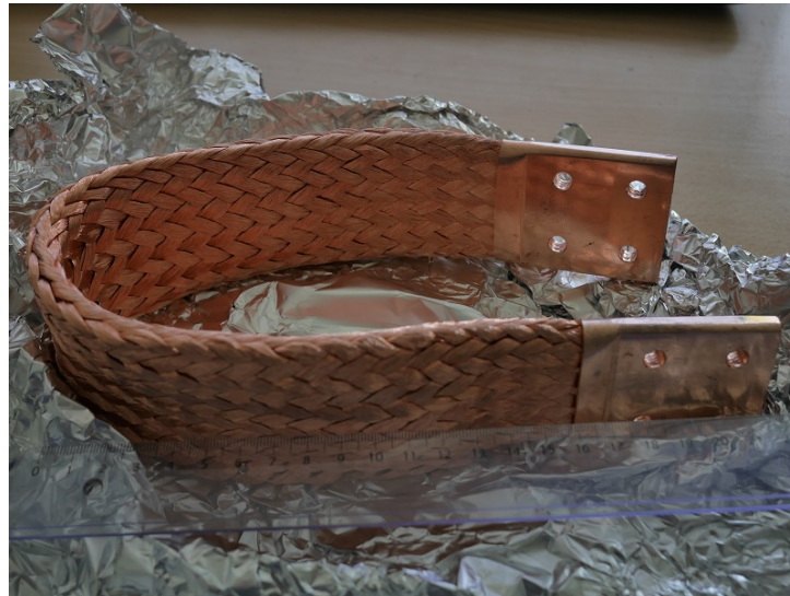
Figure 5.4: Large copper braid manufactured from electro copper with a cross-section of 210 \text{ mm}^2 [28].
