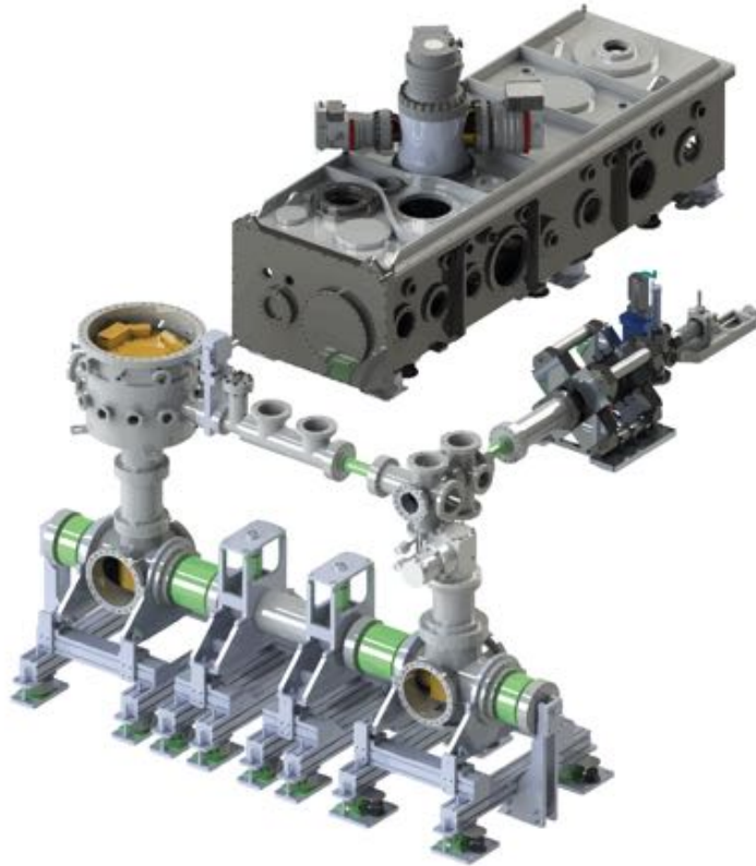
Figure 6: CAD rendering of CryPTEx II (bottom left), the beamline (bottom right), the XUV-Ebit (top right) and the XUV frequency comb (top left). Courtesy of Julian Stark.
