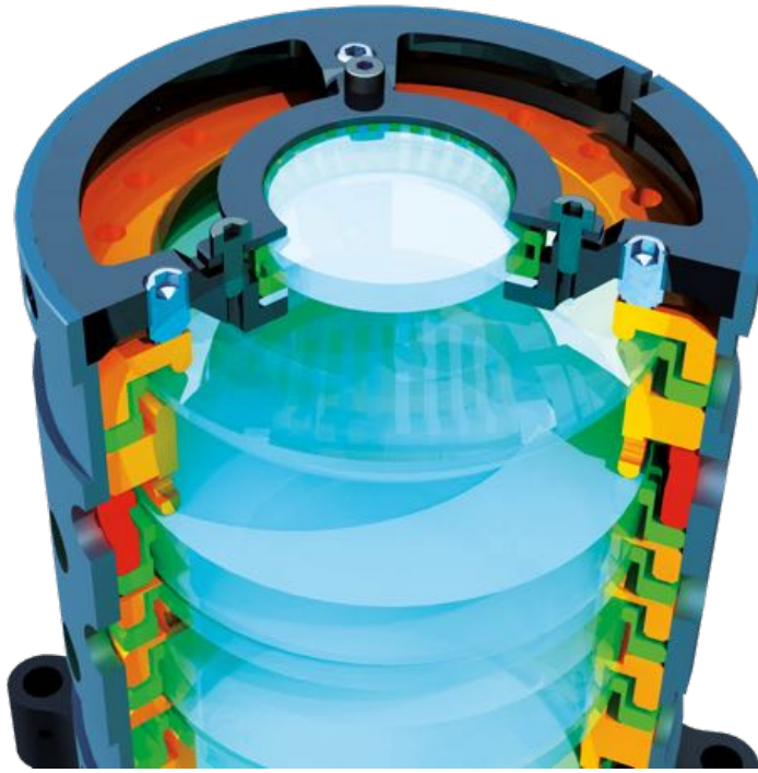
Figure 15: Illustration of the final ring (dark grey) on top of the lens stack. The anodized ring is fixed by eight M3 screws to the aluminum cage and cut by a 3 mm slit. Three arms are setting and centering the 1" meniscus lens. The mounting rings of the other lenses are pushed down by three M4 thrust pieces which are screwed into the arms.
