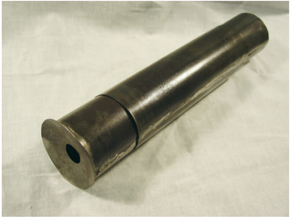
Figure 1: The first compound microscope made by Zacharias Janssen around 1606-1607. Taken from [31].
