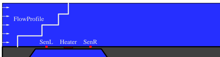
Fig. 5.9: Schematic diagram of a two-dimensional anemometer, cf. [32].
