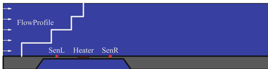
FIGURE 9 Schematic diagram of a two-dimensional anemometer, compare Reference 37.
