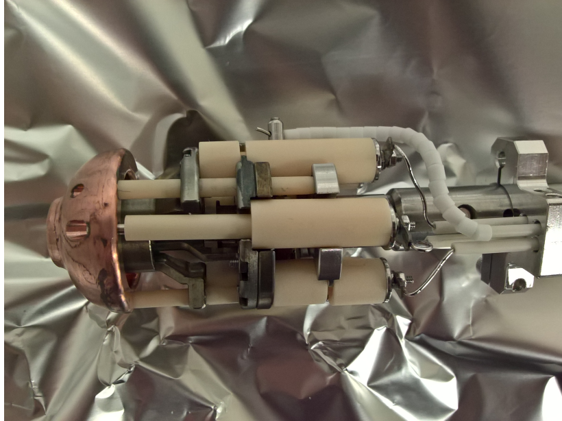
Figure 5.22: The new electron gun after assembly.
