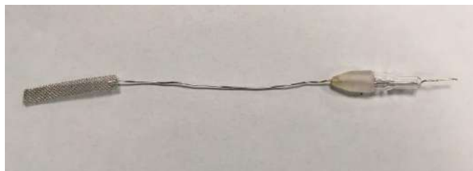
Fig. 4.3 Platinum counter electrode with a large surface area due to mesh structure.
