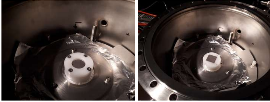
Fig. 3.11 ISOLDE sample and holder in alpha spectrometer for determining potential reduction factor caused by holder. Left : with top holder ring, right : without top holder ring
