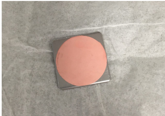
Fig. 3.13 Stainless steel plate coated using the HDPE sample holder.
